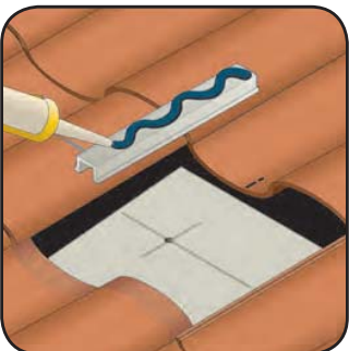
Step 5: Insert the lag bolt and washer through the TileTrac® and apply fresh compatible sealant to the base.
